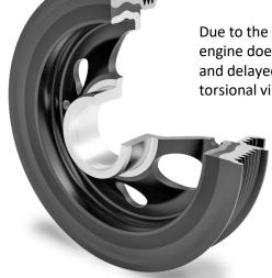
Due to the combustion cycles and ignition sequence of the cylinders the reciprocating engine does not have a perfect concentricity. The crankshaft is constantly accelerated and delayed. To counteract this characteristic behaviour, the belt pulley, also called torsional vibration damper, is used.
