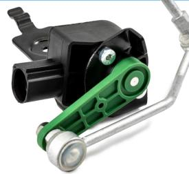
With the implementation of xenon light, an automatic headlight range control system is required by law. This regulation applies to vehicle headlights with a luminosity of more than 2000 lm, including up to date LED lighting systems.
